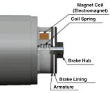
During motor operation, current flows through the magnet coil. The iron armature is attracted to the magnet coil which becomes an electromagnet when energized. As a result, the brake lining and the brake hub separate from each other, and the motor output shaft becomes free. While the motor is stopped, the coil spring pushes out the armature. As a result, the brake lining and the brake hub come into contact and hold the load.
