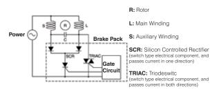
SCR is a circuit that flows the braking current. Only current from one direction flows. TRIAC is a supply circuit for commercial power. Current flows from both directions.
